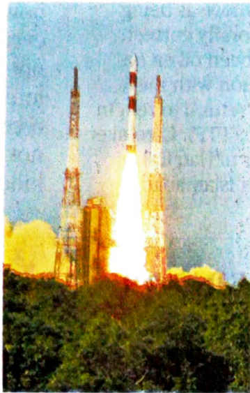
The 60th mission will employ a PSLV variant which uses two strap-on motors. FILE PHOTO
